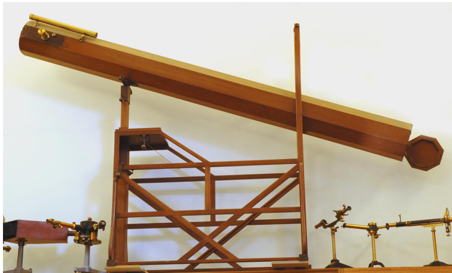
Reflecting telescope, Newtonian "Herschel Telescope", by William Herschel, English, c. 1790
