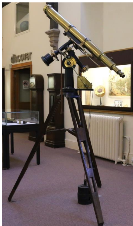
5-inch refracting telescope on an equatorial stand, with clockwork drive, 'Royal Century' model, by W. Watson & Son, English, c. 1908
